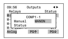
Finally, press the Enter key to make the change. In our example the relay output is now manually turned on as shown here:
