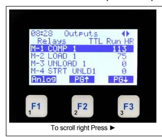
Relay Outputs TTL Run HR
