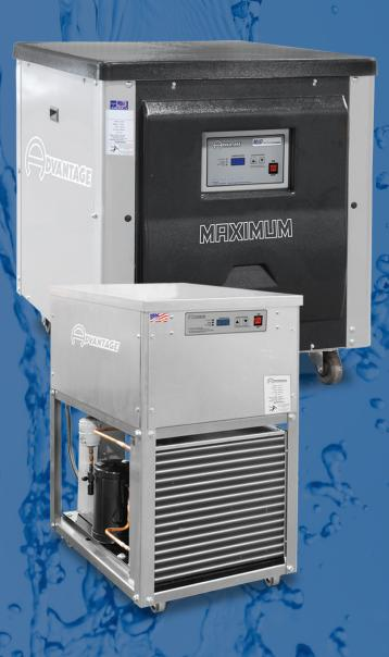
Advantage's Maximum Series Portable Chillers are refrigeration units coupled with an integral fluid circulation system that range in cooling capacity from 1/4 to 40 tons. These units are used to cool fluids to support industrial process cooling applications requiring a fluid temperature range from 20°F to 80°F.
