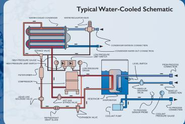
\* Water-cooled models require an external water supply source for operation.
